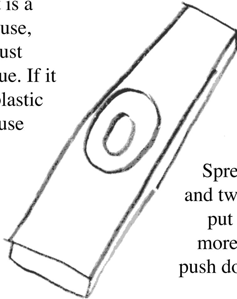
Spread it thin and even, and twist the piezo as you put it on to distribute it more. Careful when you push down on the piezo- it is very fragile!
