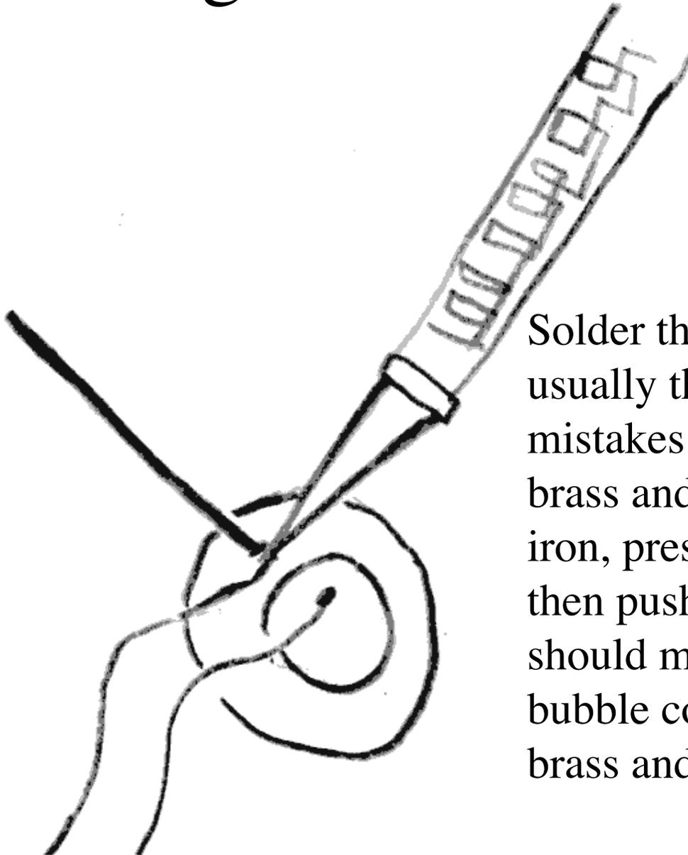
Solder the ground first because usually the brass can handle mistakes better. Touch the brass and the wire both with the iron, press for a little bit, and then push some solder in. It should molten and make a bubble contiguous around the brass and the wire.
